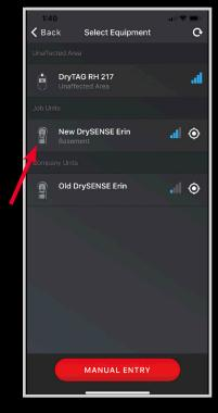
When using the DryTAG RH on a job as a standalone thermo-hygrometer, click on the affected, unaffected or HVAC. You will be shown a list of smart equipment to which the DryTAG RH can be assigned to take readings.
