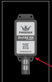
Pull out the battery tab to activate the battery
